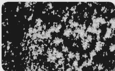
picture 15 detail of the residual dirt “glued” to the tape after the taping test on the sheet metal duct
